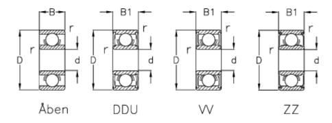
Max rpm ZZ-WW = 38000 В = 6 В1 = 6 r min = 0.3Type d = 6 =606D = 17 Load Cor (N) = 835Load Cr (N) = 2260 Max rpm DD = 34000
